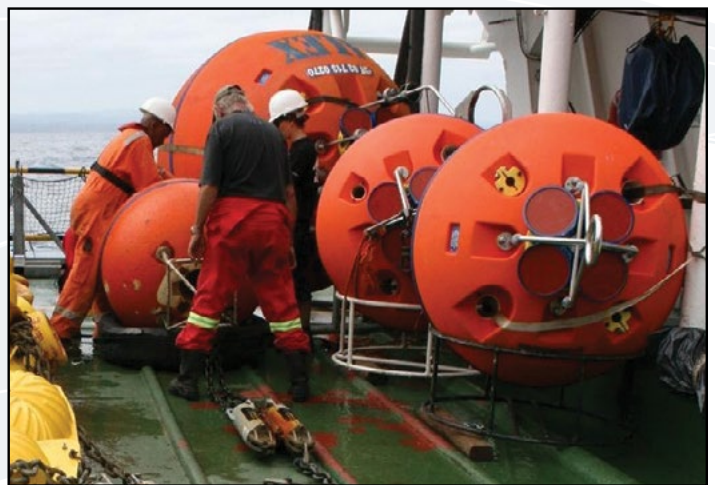
Teledyne RDI ADCPs mounted in top buoys of an ASCA mooring array.
