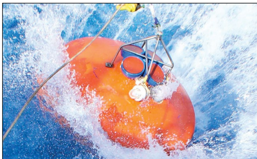
Long Ranger ADCP atop mooring for Agulhas System Climate Array (ASCA).
